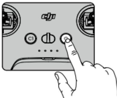
EN Press once to check the battery level.
