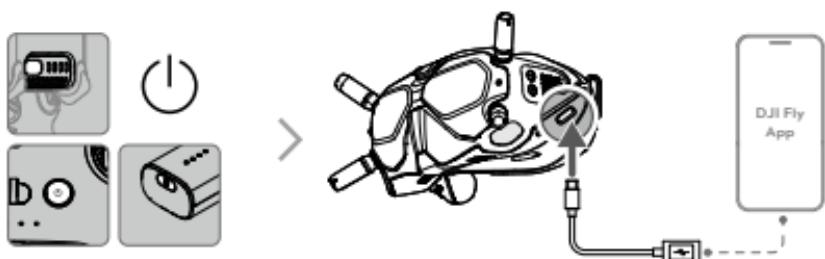
Connect the USB-C port of the goggles to the mobile device, run DJI Fly, and follow the prompt to activate.
